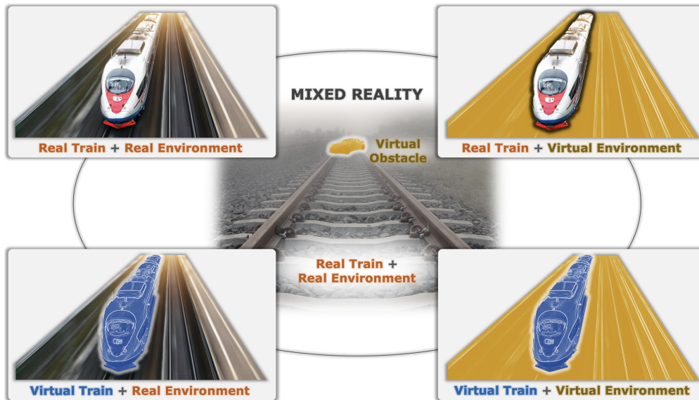
Fig. 8.1. DT-in-the-Loop and Example of Mixed Reality.
